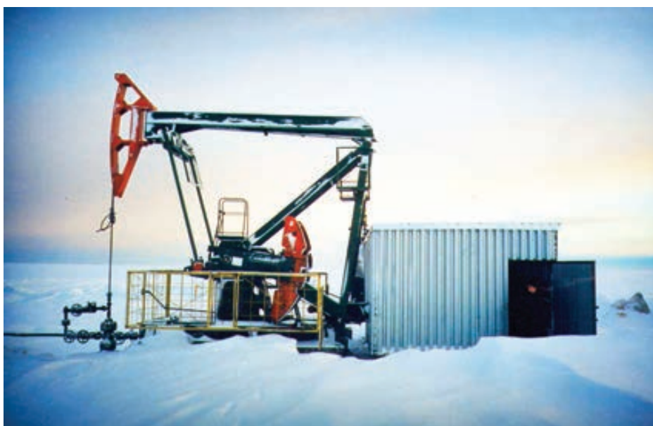
OPNSh-80 with gas engine made by OAO "Izhneftemash", Kolguev island, "Arktik-neft"
